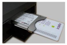
Do not attempt to use the Viewing Card/CAM in any unit except the one for which it was supplied. Cards and CAMS should never be removed unless instructed by the support team at BFBS and never touch exposed contact pads. The CAM is removed by pressing the lever at the right of the CAM slot then once it is released, pulling it straight outwards.
