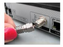
Rooms equipped for using an STB will have a cable feed with an "F type" screw connector. Ensure the centre conductor protrudes slightly as shown below, guide it into the dish connector on the rear of the STB and screw it in place.
